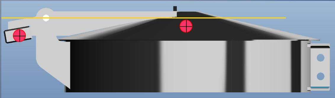
The counter weight CG and lid CG were optimized by placing them below the pivot axis instead of on the same plane as the pivot axis. With most other product, the closing force approaches zero as the lid opening angle approaches 90 deg, therefore the lids only open to a smaller angle in order to maintain a closing force.
