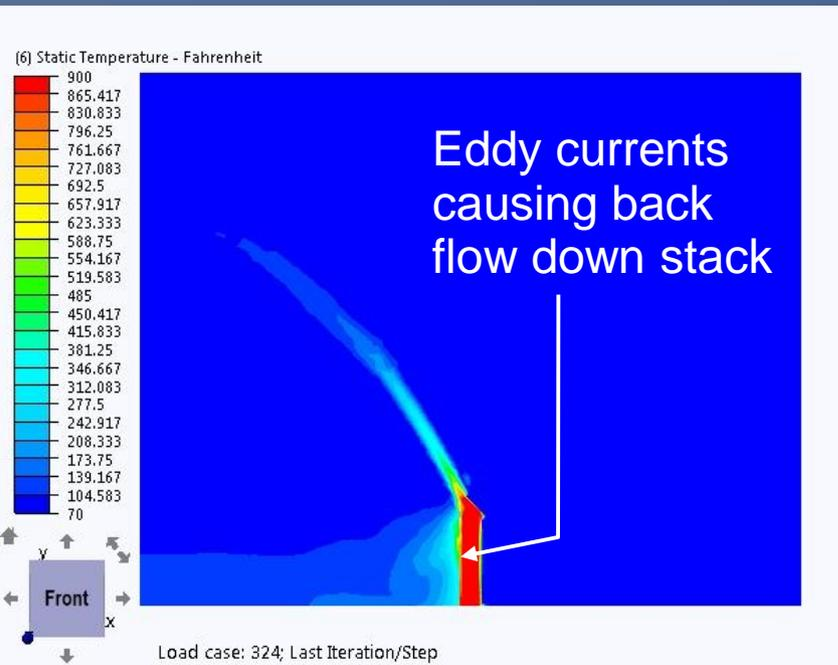
The bottom analysis is a 5 ft long stack with a rain cap at 45 deg in a 10 knot wind from the right. Note the eddy currents and back flow down the stack. This can cause exhaust fumes to cycle back to the enclosure or into ground level surrounding areas.
