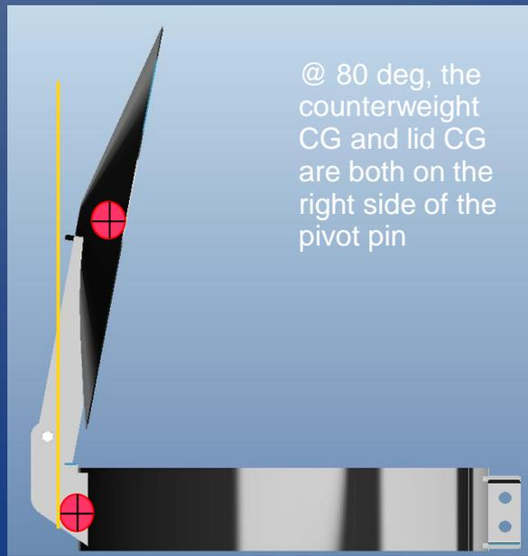
@ 80 deg, the counterweight CG and lid CG are both on the right side of the pivot pin
