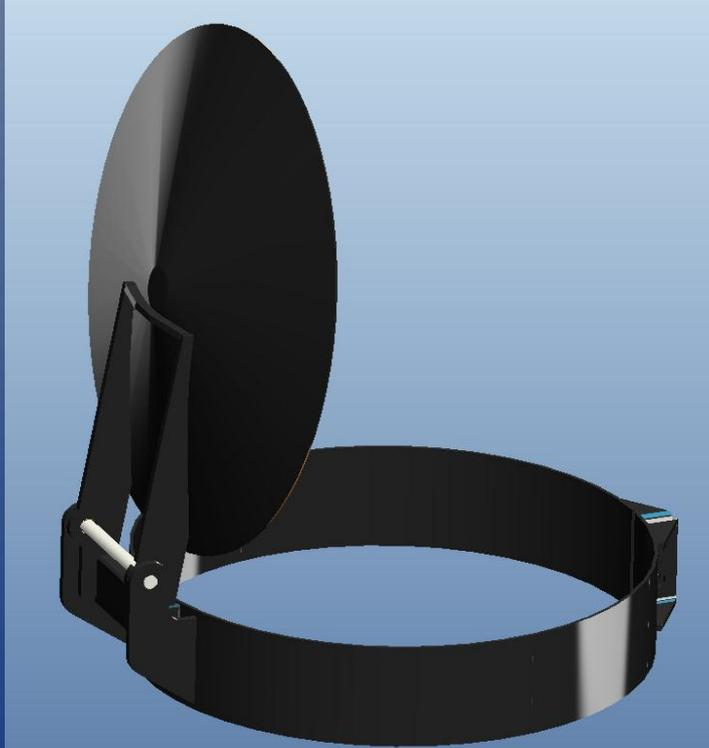
The larger opening angle also reduces the impact force at the opening stop point during a backfire event. The backfire force has less surface area to act on and a less effective force vector angle.
