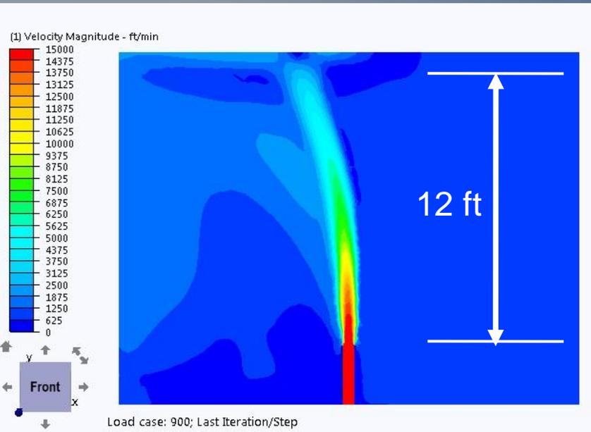
The top analysis is a 5 ft long stack without a rain cap in a 10 knot wind from the right. Even in the wind, the exhaust flows straight up. This is the desired effect if the rain cap was present.
