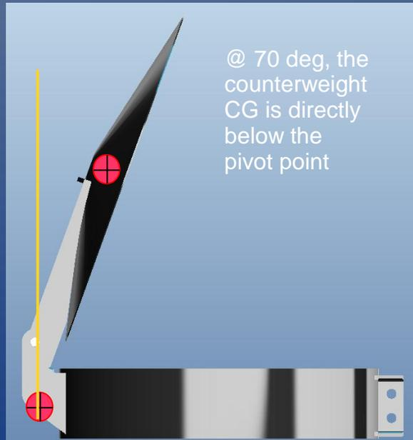
@ 70 deg, the counterweight CG is directly below the pivot point
